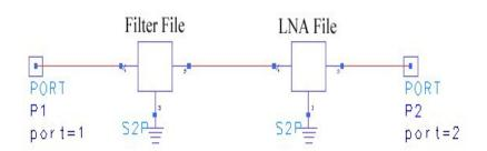
• Network measurement of Filter/Amplifier
